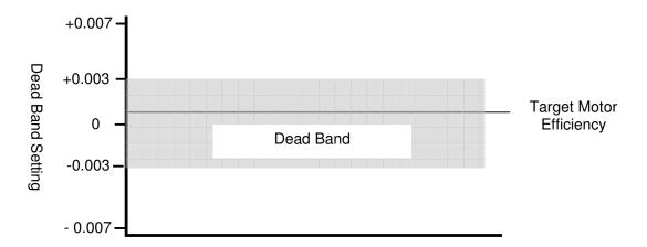
The Dead Band is the area above and below the target efficiency (See Optimum Efficiency) in which Powerboss will not react to a change in motor loading, thus creating a 'Dead Band' to ensure system stability.
