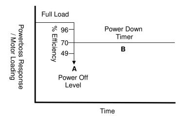
The Timed Power Off feature is useful for applications that run at no load for prolonged periods of time, such as a Mechanical Press. Powerboss can be programmed to recognise the no load period and switch the motor off. Powerboss will still provide Optimisation until the motor is switched off.
