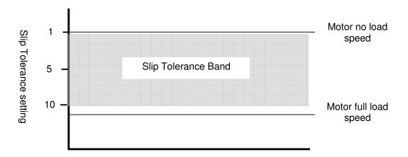
The Slip Tolerance Setting will allow the motor to slow down to a set point during a no load condition before any Stall Compensation can take place. This feature allows a higher level of Optimisation during periods of no load on high inertia applications such as a flywheel press.
