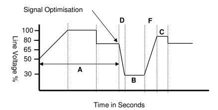
The Signal Optimisation feature is useful on applications with a cyclic load, such as a Circular Saw in a Sawmill. To use this feature a normally open, volt free, contact from a sensor needs to be connected into terminals 5 and 6 on terminal block TB1.
