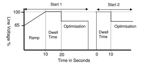
If the above application is selected a DOL start can be selected (Start 2) by bridging terminals 3 and 4 on Terminal Block TB1. This feature is useful should a full toque start be required if the Crusher must be started when loaded.
