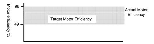
The Optimum Efficiency Setting dictates the point at which Powerboss will attain full voltage during the motors load cycle. Powerboss will automatically try and adjust Actual Motor Efficiency to the set Target Efficiency.
